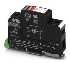
Surge voltage arrester consisting of base element with remote indicator contact and ground connector with high-capacity varistor, for mounting on NS 35/7.5, nominal voltage: 230 V AC, 1-channel
